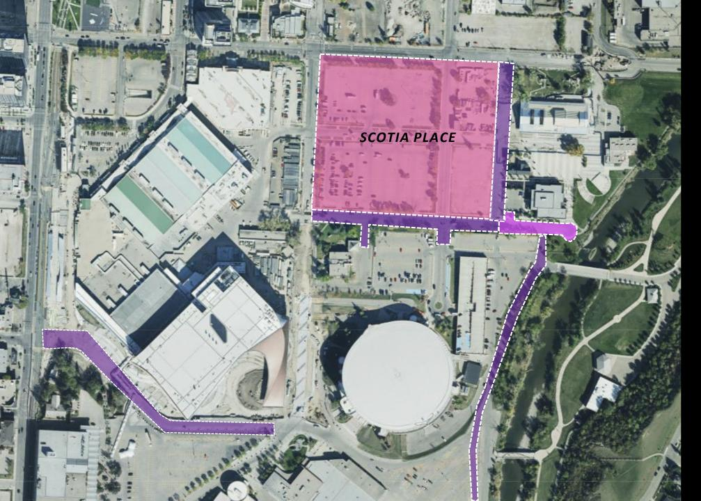
**5A Street SE:** Relocation of 5th Street SE to a new location east of the CEC parcel providing a minimum 4-lane cross section with lane reversal between 12th Avenue and 14th Avenue SE.
